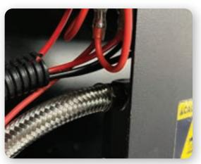
Once the compressor is operating, air is moved from the compressor into a 2.5-gallon tank via braided air hose pictured above.
