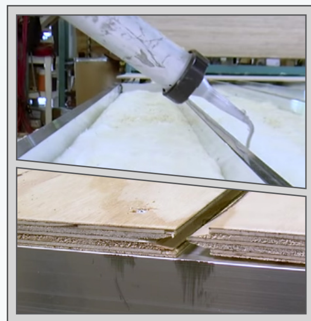
GLUED & SCREWED PLYWOOD FLOORING 5/8" Tongue and Groove Plywood Floors that are Glued & Screwed on 1" x 3" Aluminum Floor Joist 16" on Center with Forced Air Heated and Enclosed Underbelly (3/4" Marine-Grade Composite Floor Decking on KTH Toyhauler)
