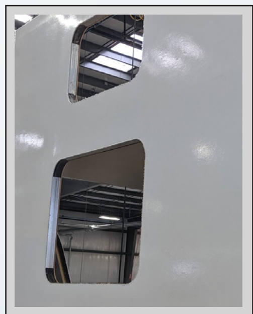
FULL FRAMED ALUMINUM OPENINGS All Windows, Doors, and Access Panel Openings Fully Framed in 2" Aluminum on TT & KTH (1 1/2" on LE) (3" on Xtreme 365)
